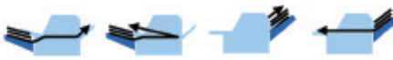
A stack of sheet With Cut Sheet Feeder and Rear Stacker *some paper paths require optional accessories
